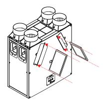
4. Filters should be replaced every two years, or after three cleaning cycles. Contact Vent-Axia Sales by calling 0844 856 0590 quoting the model reference.
