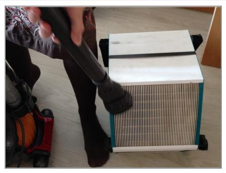
Clean the cell on each side with a hoover to remove any dust
